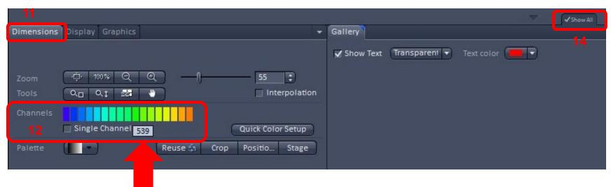
15. You can turn off any channels you want by clicking on the colored bar that represents that channel. In this example the 504 and 584 channels were turned off.
