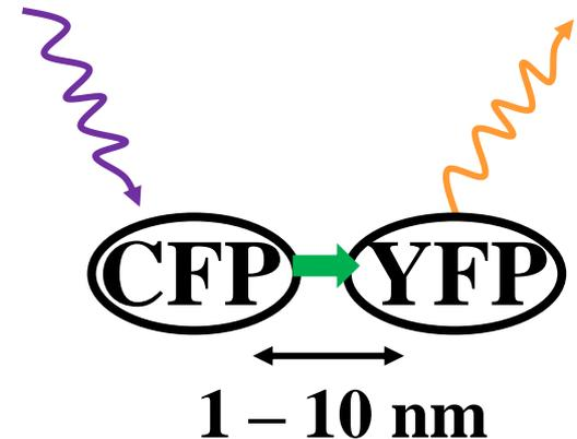
This is another example of FRET. In the reduced linker the ECFP and EYFP are more than 10nm apart so excitation of ECFP will not excite EYFP so we get a Green signal. When the linker is oxidized it brings the two closer and we have FRET or Red Signal.
