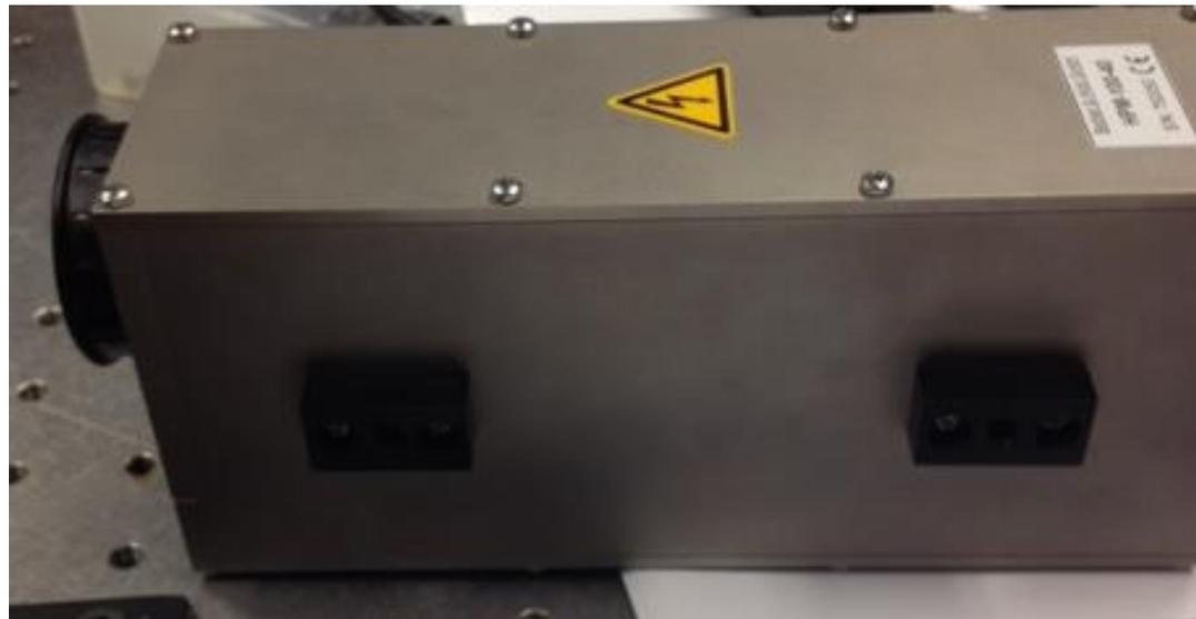
11. Carefully loosen the screws of the cover and remove the cover.
