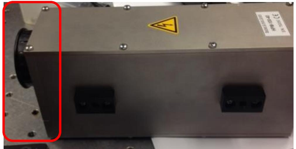
**62. Replace the cap on the NDD detector.**
