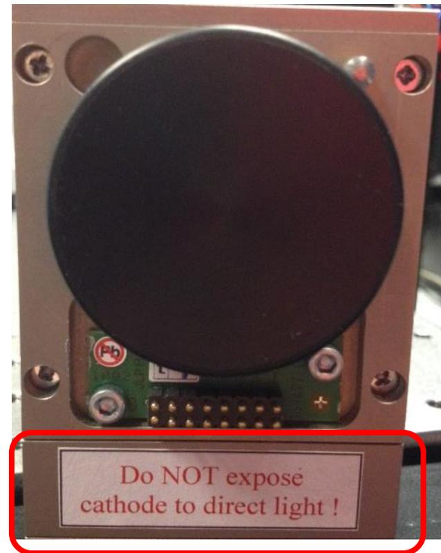
15. This is how the FLIM Detector looks when attached to the NDD.
