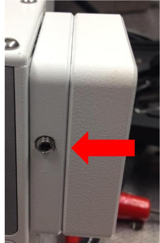
12. Be aware of the laser safety interlocks. They are located on the inside of the cap as well as the NDD. If they are not secured in place both with correct pin alignment and tightened with the screws the lasers will not fire.
