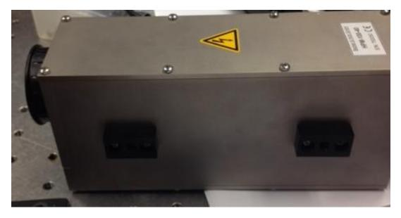
11. Carefully loosen the screws of the cover and remove the cover. Do not let the screws fall off the NDD.
