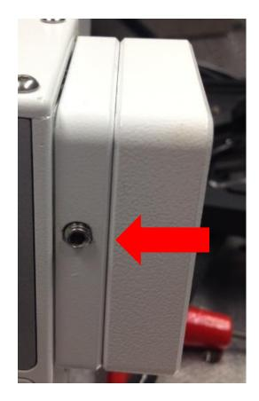
12. Be aware of the laser safety interlocks. They are located on the inside of the cap as well as the NDD. If they are not secured in place both with correct pin alignment and tightened with the screws the lasers will not fire.
