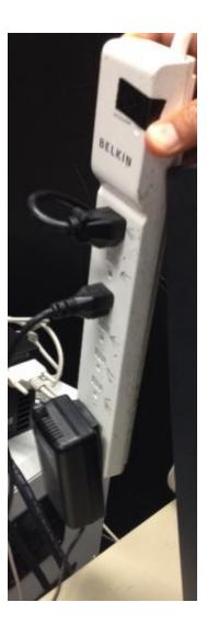
16. Locate the power strip behind the FLIM Monitor and turn the power switch on. The Power Switch is located at the side of the power strip.
