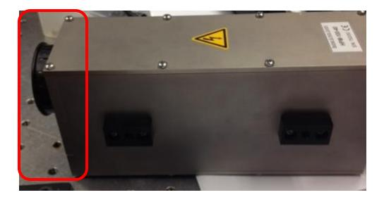
62. Replace the cap on the NDD detector.
