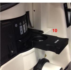
Step 14: Using the silver aperture diaphragm knobs on each side to adjust octagon to center.
